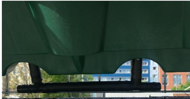
Join these sections together with 13mm pipe and lead the overflow water away to a drain or Back to a feed tank. (Depending on size and design of system)
